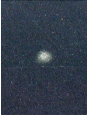
A stone bruise is a white, discolored area of stone caused by a direct blow of some sort. The natural color of the stone is caused by the particular way it absorbs and reflects light. When a part of the stone is damaged by a hard blow, the crystal lattice that makes up the stone is deformed, and it changes its optical properties. Now it reflects more light - instead of absorbing some - and turns white.
