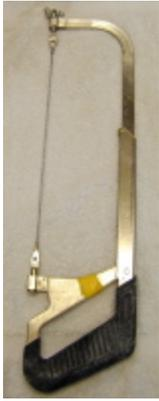
A more durable saw - that will cut even harder stones with patience - is made for cutting tile. The tile cutting blade we have is made of an abrasive grit adhered to a steel wire. It fits into a standard hacksaw and will cut just about any stone we want. Because of the design of the blade it cuts on both the push and the pull, but the teeth are very small, so cutting isn't particularly quick.
