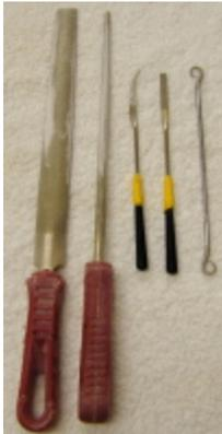
Diamond files come in various shapes and sizes. Like structured carbide they cut in any direction. Since diamond is so expensive you won't find big, course files made with it. As a result you'll generally use diamond files in limited situations - to do finer shaping - generally on hard stones.
