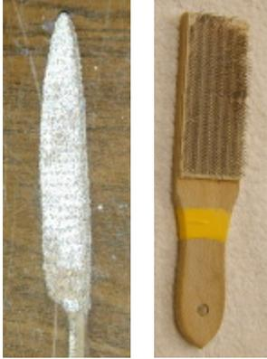
Sometimes - depending on the nature of the stone and the shape of the teeth of the file you're using, the file will "load" with dust, as shown here in a structured carbide file in the image on the left.
