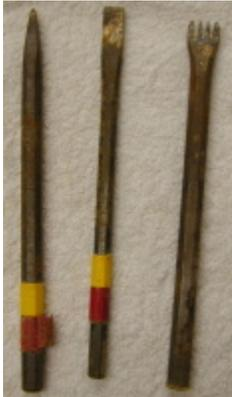
The most commonly used chisels on our recommended starter stones are toothed and flat chisels. See the larger discussion about chisel types below for more details, but if you get one or two toothed chisels and at least one flat chisel, you're probably fine. Beginner's kits usually include a point chisel as well, but on smaller, soft stones it isn't often needed. You'll use it later on larger and/or harder stones, though, so it isn't money wasted.
