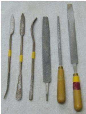
Structured carbide files are very durable and cut stone in any direction. (That is, they remove stone on both the push and the pull. They can even be used with a sideways motion.) They also work on very hard stones. Highly recommended, and even more durable than Italian stone files, but not available in as many shapes and sizes.
