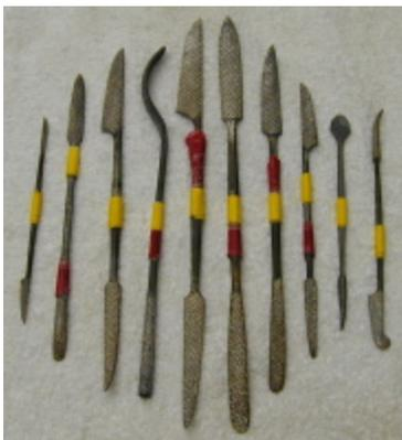
These are Italian stone carving files. They have very evenly spaced teeth and are properly hardened to work well on stone, even on most marbles. They are generally only available from a stone carving tool supplier.
