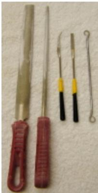
Diamond files come in various shapes and sizes. Like structured carbide they cut in any direction. Since diamond is so expensive you won't find big, course files made with it. As a result you'll generally use diamond files in limited situations - to do finer shaping - generally on hard stones.
