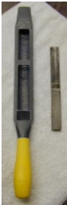
These are common files that might be purchased at a hardware store. Neither is particularly expensive, and all will work on soft stone. The one on the left is a Sureform 21-295 file made by Stanley, with a curved file blade replacing the usual flat blade. (We've generally found more use for the curved blade in this file.) The one on the right is a common four-in-hand.
