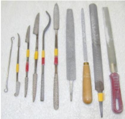
Files (also called rasps and rifflers) are used to remove small amounts of stone. They can remove marks left by chisels, and can bring a sculpture to its final shape before polishing. Usually made of steel, there are many, many shapes and sizes available. Most files sold in common hardware stores are intended for use on wood. These will generally work on soft stones, but will not work well on anything reasonably hard, like marble.
